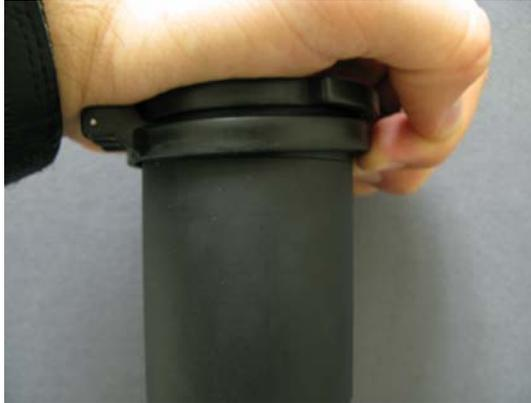
2. Once the edge of the cover is over the ridge in several places, it should easily come off exposing the ridge that goes around the finish ring.
